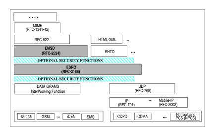
Figure 1: LEAP Protocol Stack
