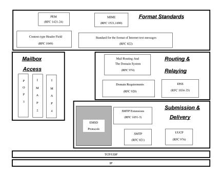
Figure 4: Messaging Communication Stack and EMSD
